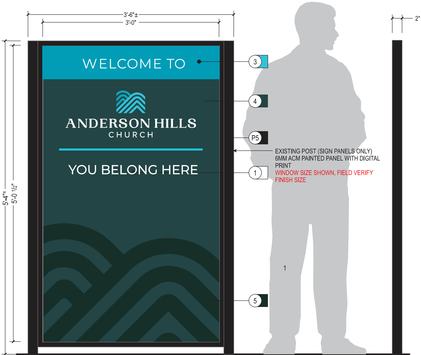
1 WF06: ELEVATION & SIDE MATERIALS: --- VERIFY MEASUREMENTS PRIOR TO FABRICATION/INSTALLATION EXTERIOR SIGN PACKAGE: PEDESTRIAN DIRECTIONAL 1" = 1' - 0"
